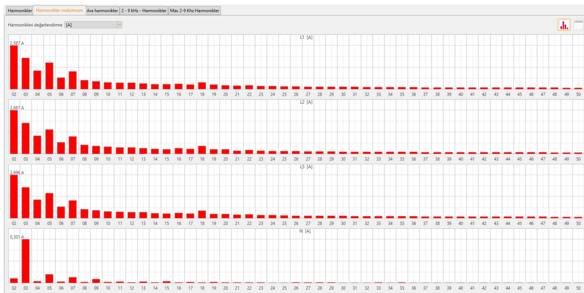
Figure -11: Spectrum of Current Harmonics from 2nd to 50th Degree
