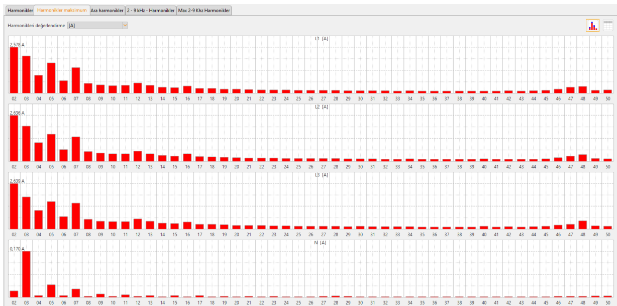
Figure -6: Spectrum of Current Harmonics from 2nd to 50th Degree
