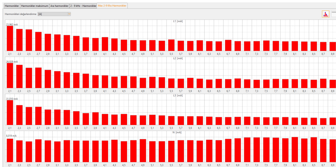
Figure -12: Spectrum of Harmonics in High-Frequency Current
